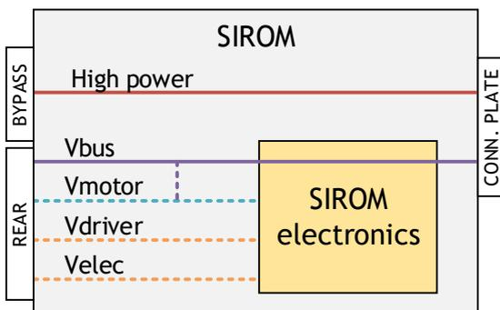
Figure 2: Power supply functional diagram
