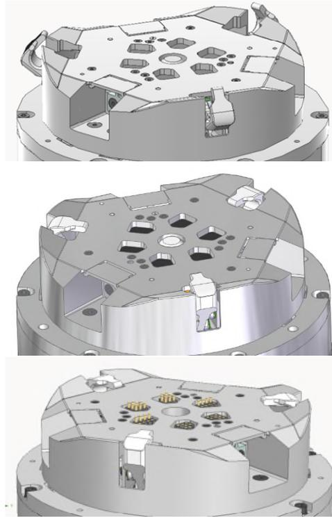
Figure 1: Latching operation, from RTC (up), LAT (middle) and CON (bottom)
